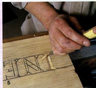
Three basic hand positions are shown here as Cushwa sets in and makes two vertical straight cuts for an I. Some trimming with the skew completes the letter.
