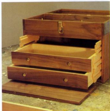
The drawers, which will be lined with adhesive-backed felt, ride on moving slides that allow full extension. The drawer-cover panel stows away beneath the bottom drawer when the chest is in use.
