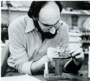
Glenn Braun attends to the yards on a tiny ship prior to mooring her inside a bottle. Hinged masts fold flat to fit through the bottle's neck.
