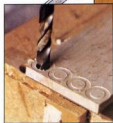
After the coves are laid out with a plug cutter, the pin holes are bored with a twist drill.
