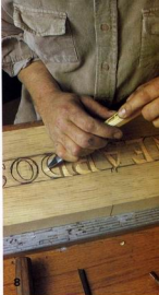
Rough out the inside and outside arcs of curved strokes with a skew before slicing around the outside curves with a gouge.
