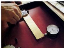
To ensure the accuracy of each of his squares to 0.002 in. over the length of the blade, Economacki devised the dial-indicator jig shown here. Referenced against the steel pins, the square's angular error is converted to a directly readable linear run out.
