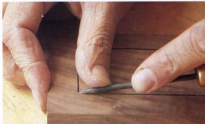
Pine stops the grinder cut just short of the intersection of the two grooves to avoid marring the wood outside the inlay border, then connects the grooves with a \frac{1}{16} -in. chisel ground from a file, above. Inlay corners look best mitered. Pine eyeballs the miter angle, using the corners of the inlay grooves for reference, then scores the stripe with a skew chisel, top right. He cuts the strip on a small hardwood block, making a bevel cut to size the piece, then paring down to the line.
