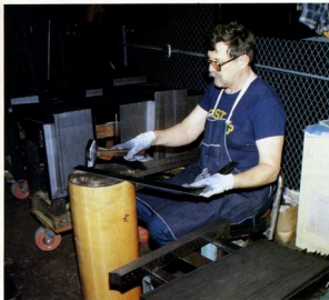
Stanley's best carpenter's squares are hand-hammered to tolerances of 0.005 in. in 15 in. of tongue length. Lew Levine first flattens the tongue on an anvil of end-grain maple, above. Then he trues the square by hammering it as shown in the drawing. A dial-indicator setup similar to Economaki's measures run out. Abrasives (right) play an important role in squaremaking. After the blades are riveted at Stanley, they're sanded flush and sharp metal edges are eased on a large belt sander.
