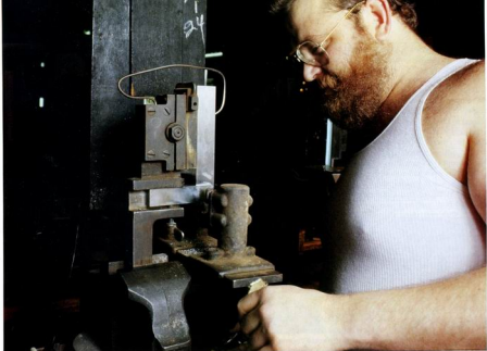
At Starrett, blades are soldered not riveted to the beams. Scott Songer, above, heats both sides of the beam with a dual-tip burner then feeds solder in as the joint warms. Once soldered and quenched, he tests the soundness of the joint by gently tapping the flat of the blade on his vise. A bright, tuning-fork ring indicates a good joint and the square is ready for testing.
