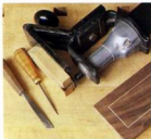
A tool-and-die makers' rotary grinder, left, mounted on shop-built stand cuts the inlay grooves. Shaped blocks can be attached to the 6-in. by 3-in. stand to guide the tool against a fence or curved template. To cut ⅛-in. slots for inlay, Pinz mounts a small Dremel circular saw in the grinder. The wooden block around the blade sets the depth of cut, and the base of the stand bears against the edge of the piece being cut.
