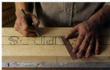
Frank Cushwa carves a sign (top) with only a skew chisel and a few gouges. His waist-high bench, its surface about 2½ ft. on a side, allows him to move around large signs. Cushwa lays out letters freehand (bottom), using a plastic rule for straight lines. Spaces between letters should be roughly equal in area.
