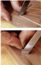
Pine stops the grinder cut just short of the intersection of the two grooves to avoid marring the wood outside the inlay border, then connects the grooves with a \frac{1}{16} -in. chisel ground from a file, above. Inlay corners look best mitered. Pine eyeballs the miter angle, using the corners of the inlay grooves for reference, then scores the stripe with a skew chisel, top right. He cuts the strip on a small hardwood block, making a bevel cut to size the piece, then paring down to the line.
