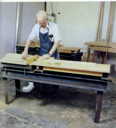
T.H. Ralph's sliding-table crosscut saw has 9-in. travel and will saw stock up to 2½ in. thick. The Thomson linear-motion bearings, visible in the photo at near right, ride on a 1½-in. precision-ground shaft mounted in a pair of steel supports. The sliding table's outboard end rolls on a wheel cannibalized from garage-door hardware. Its bearing surface (photo at far right) is a piece of heavy angle iron that can be raised or lowered to square the table to the blade in the horizontal plane.
