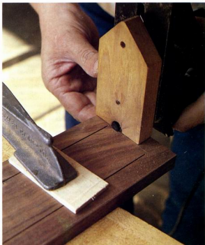
A tool-and-die makers' rotary grinder, left, mounted on shop-built stand cuts the inlay grooves. Shaped blocks can be attached to the 6-in. by 3-in. stand to guide the tool against a fence or curved template. To cut ⅛-in. slots for inlay, Pinz mounts a small Dremel circular saw in the grinder. The wooden block around the blade sets the depth of cut, and the base of the stand bears against the edge of the piece being cut.
