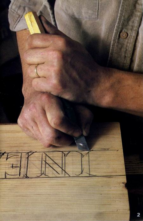
Three basic hand positions are shown here as Cushwa sets in and makes two vertical straight cuts for an I. Some trimming with the skew completes the letter.
